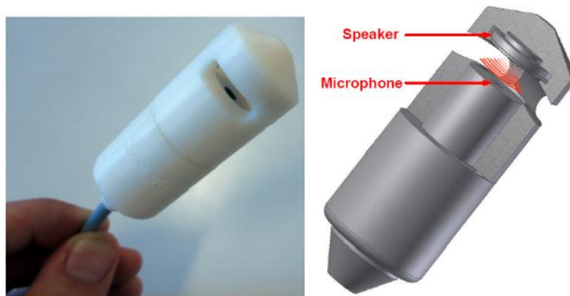
Figure 14 - The self-testing noise measurement sensor developed in IDEA [23].
