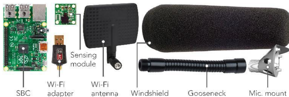
Figure 18 - Main part list for complete node at relative scale (SONYC) [28].
